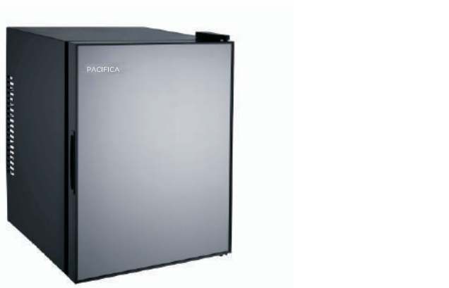
PCF044-04 Minibar Mute semiconductor refrigeration Capacity:36L Size:380x445x475mm Net weight:11kg Cooling Temperature:5-8°C Voltage:220-240V (50-60Hz)/110-120V(60Hz) Energy consumption:0.75(KWH/24H) Intelligent automatic defrost system Door controlled LED light Reversible door opening direction 100% green & HSF(Hazardous Substances Free)
